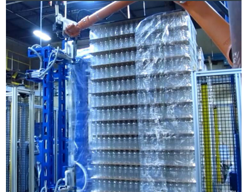
Robot unwrapping pallet of PET bottles
