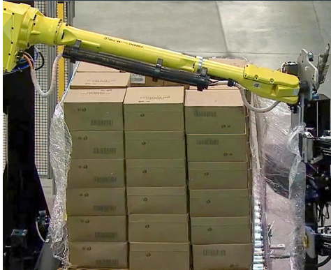
Robot unwrapping pallet of cased product
