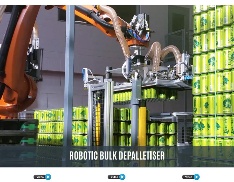
Goldco's state-of-the-art Robotic Bulk Depalletisers are specifically designed to efficiently handle a wide range of product sizes from numerous incoming product lines, seamlessly delivering them to many distribution lines. With the flexibility of different end-of-arm tooling options, our depalletisers are capable of effortlessly depalletising both empty and filled cans (aluminium or steel), plastic containers, as well as cases.
