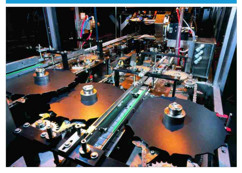
BW Integrated Systems' **T I S M A Series** WrapStar Sleever sets the standard for sleeve packaging productivity utilizing robust construction and multi-axis servo technology. The WrapStar Multiwrap Sleever features continuous motion functionality and handles a wide variety of product shapes.
