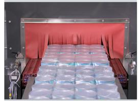
Shrink-wrapped trays exiting the heat tunnel
