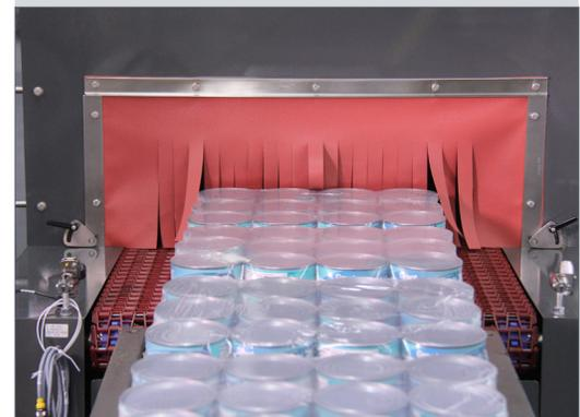
Shrink-wrapped trays exiting the heat tunnel
