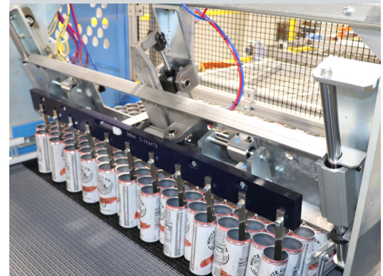
Staggerhead assembly forming can pattern
