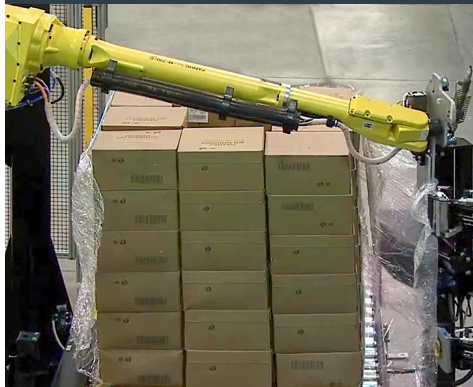
Robot unwrapping pallet of cased product
