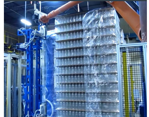
Robot unwrapping pallet of PET bottles
