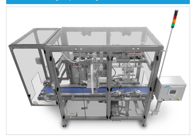
BW Integrated Systems' fully automatic Series 1579 High-Speed Uncuffer / Closer uncuffs a filled polyethylene bag from a corrugated case, gathers the bag, and applies a polypropylene tape or plastic clip closure to the neck of the bag.
