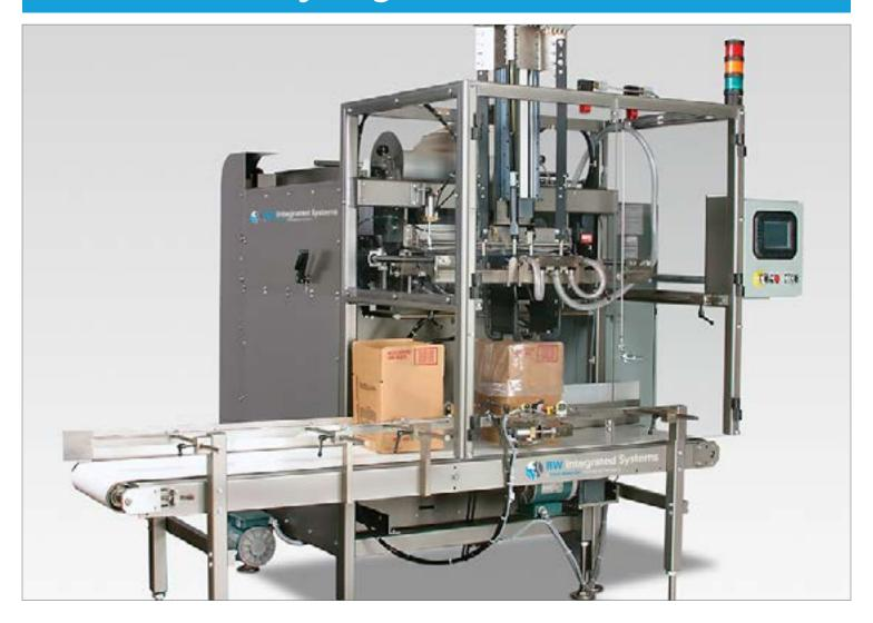
BW Integrated Systems' fully automatic Series 1575 Poly Bag Inserter is designed to select a gusseted or flat tube polyethylene bag from a roll of perforated stock, insert it into an erected container (corrugated, plastic, etc.), and cuff the top over the container flaps.
