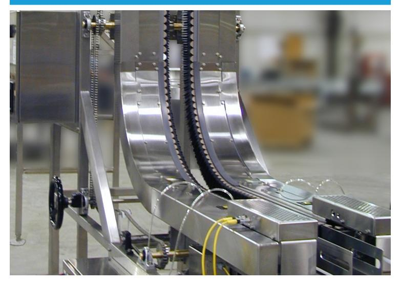
BW Integrated Systems' Elevator / Lowerators raise or lower containers with ease. When significant elevation changes are required in your bottling line, our gripper elevators or lowerators are your best choice.
