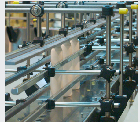
Baseblow Air Conveying
