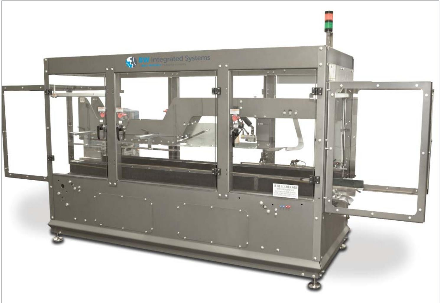
BW Integrated Systems' SWF CS 430 Case Sealer is a rugged, highly efficient and versatile case sealer. It can be configured and manufactured to seal with either tape or optional hot melt glue. Changeover is simple with hand cranks or levers so that no tools are required. Cases are transferred through the sealer with side belts to allow positive transfer and maintain square flap sealing.
