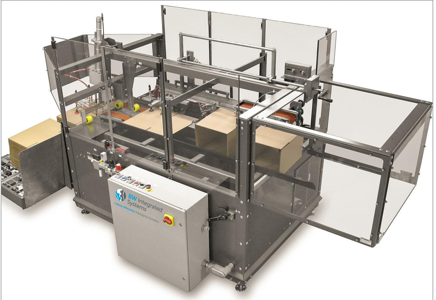
BW Integrated Systems' Thiele CE 446 Case Erector automatically selects, erects, squares and seals the bottom flaps of regular-slotted (RSC), and half-slotted (HSC) corrugated cases. Speeds of up to 20 cases per minute are possible, depending upon the model configuration and case size.
