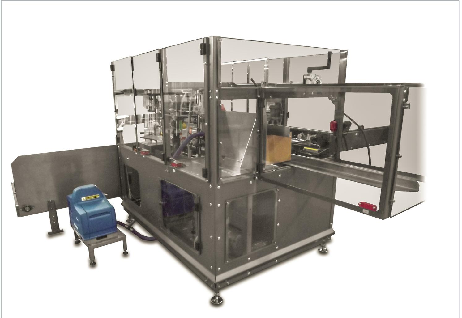
BW Integrated Systems' Thiele CE 442 Case Erector automatically selects, erects, squares and seals the bottom flaps of regular-slotted (RSC), and half-slotted (HSC) corrugated cases. Speeds of up to 30 cases per minute are possible, depending upon the model configuration and case size.
