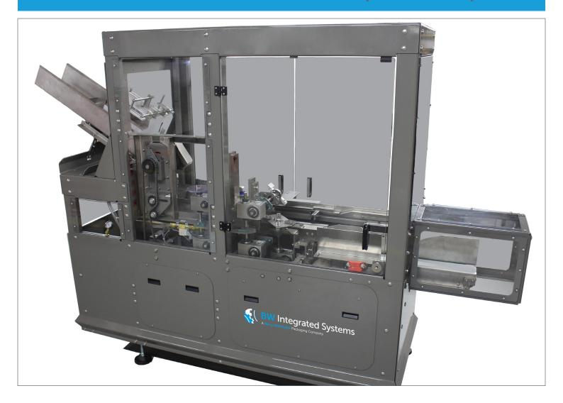
BW Integrated Systems' **SWF Series** BCE 46 Basket Carrier Erector automatically selects, erects, and locks the bottom of four to six pack basket carriers. This machine is equipped with a three-foot long, inclined magazine for loading the basket carrier blanks. An extended horizontal magazine is available, increasing the time between refilling.
