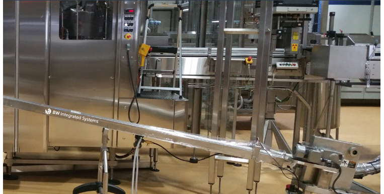
Fleetwood Manual Can Lid Feeder with LLV Low Level V-Tray in production
